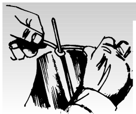
Form loops in coat hangar wire. Bend the wire around a small nail held in a vise.
